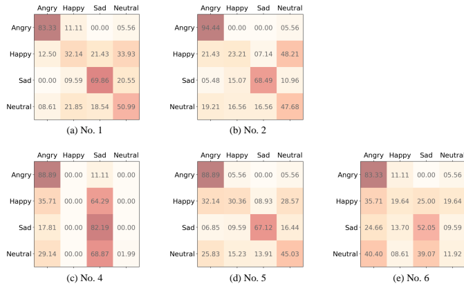
Fig. 3. Confusion matrices of systems in Table II when tested on IEMOCAP. The numbers in the cells represent the percentage that a ground-truth emotion (row label) is recognized as a particular emotion (column label).
